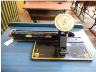
A dial typewriter which is a child's typewriter but resembles the Columbia Index machine (1885). The handle on the dial controls character selection.
